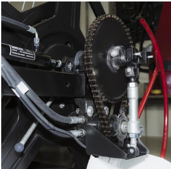
The hydraulic reel drive
