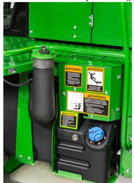
Fuel and diesel exhaust fluid tanks
