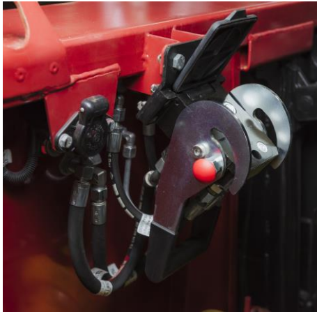
Single-point hydraulic coupler
