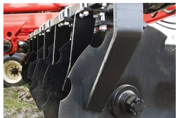
Wear-resistant disc scrapers
