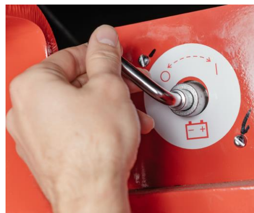
Battery disconnect switch
