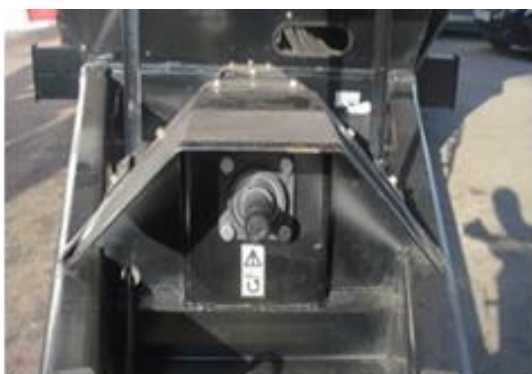
Direct worm drive from tractor PTO
