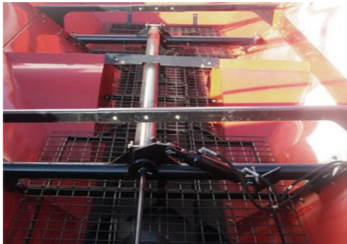
Valves inside the grain chamber
