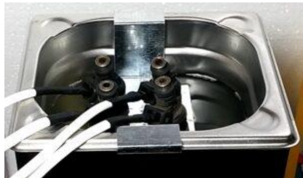
Washing the injector in the ultrasonic bath
